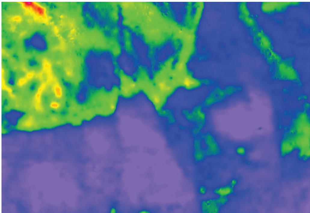
Ground Conductivity Mapping is one of the most cost effective Geophysical methods available. Rapid acquisition is made possible using custom vehicle setups (using a 4WD or ATV). Ground conductivity and position data are logged continuously in real-time whilst driving, making it possible to cover many hectares in one day.
